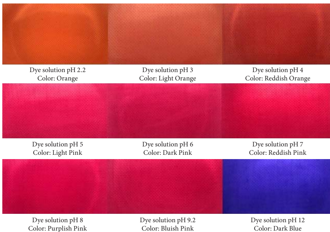
Figure 8: Colour change of cotton fabric dyed with synthesised dye in different pH solutions
