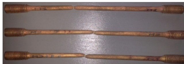
Fig. 4 Specimens after uniaxial tension test
