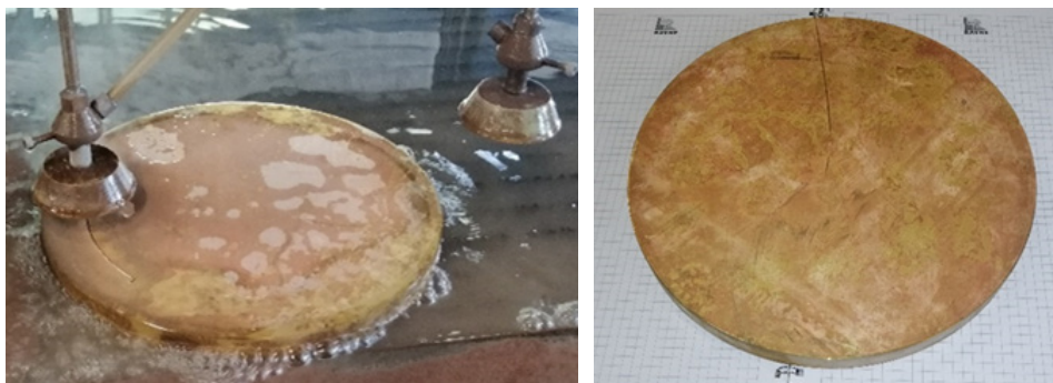
Fig. 7 Cutting the blank by the water-jet process (left) and the blank after chemical treatments (right)
