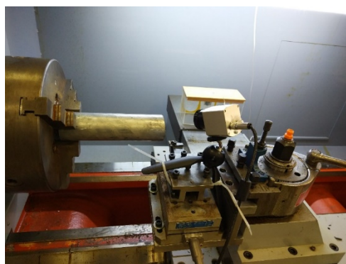
Fig. 1 Experimental setup for MMC turning with thermal imaging camera
