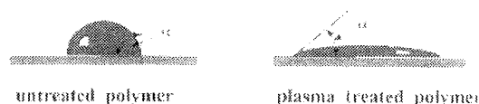
Measurement of surface tension (polar and dispersive) by measurement of contact angles of different liquids on a treated surface
