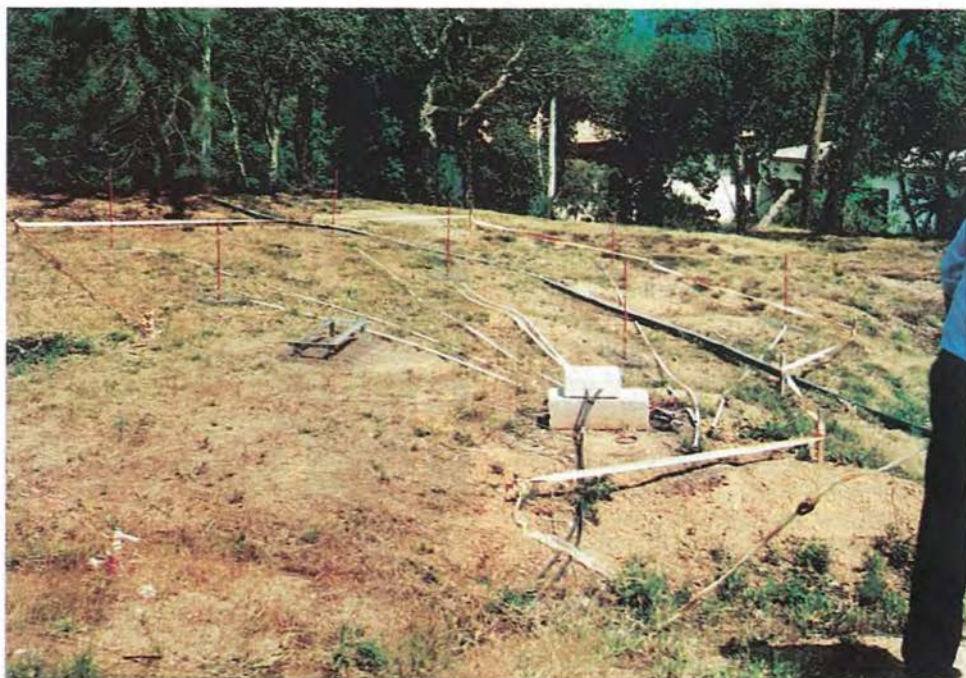
Slika 3. Merjenje sušenja in vlaženja mrtvega kuriva iglic primorskega bora (foto: T. Dimitrov) Figure 3. Drying and Wetting Measurement of the Needles' Nonliving Forest Fuel of the Littoral Pinus nigra dalmatica
