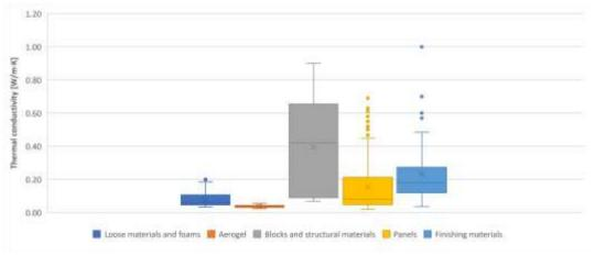
Figure 10: Thermal conductivity of the building thermal insulating materials
