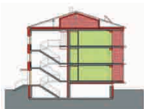
Slika 5: Področja renovitvenih posegov: prerez (Dornbirn). Vir: Task: 37, Architecturbüro Kuess, www.iea-shc.org/task37 Figure 5: Areas of renovation interventions: cross-sectional view (Dornbirn).
