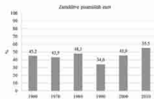
Graf 4: Odstotki zasteklenih površin na fasadah pisarniških etaž vzorca analiziranih visokih poslovnih stavb v Sloveniji po dekadah od leta 1960 do danes. Graph 4: Percentages of glazing on the facades of office units calculated on a sample of high-rise business buildings in Slovenia in decades from 1960 onwards.
