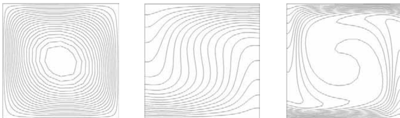
Figure 2. Streamlines, isotherms and isoconcentrations for A = 1 , Ra = 100 , Da = 10^{-4} , Le = 10 , N=0.2 .
