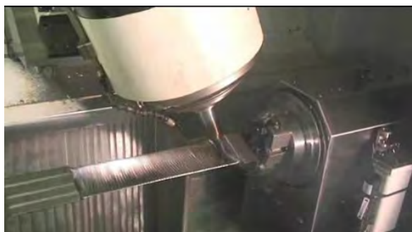
Fig. 4. Machining process of the turbine blades
