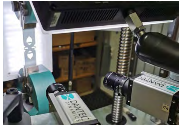
Fig. 9. Image acquisition using a backlight
