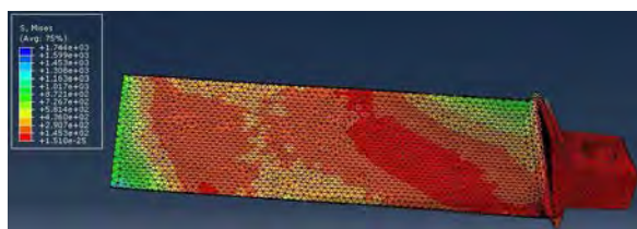
Fig. 7. The calculated residual stresses by the Von Mises yield criterion due to machining operation of turbine blade in MPa unit
