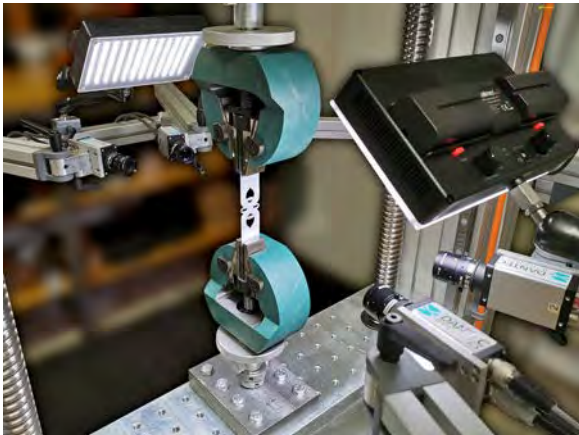
Fig. 8. Measuring setup utilizing the digital image correlation
