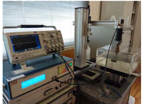
Fig. 6. Experimental setup for attenuation evaluation
