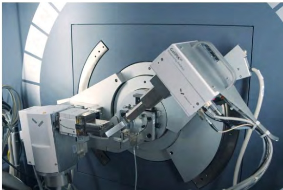
Fig. 9. The X-ray diffraction method to measure the residual stress of machined turbine blade
