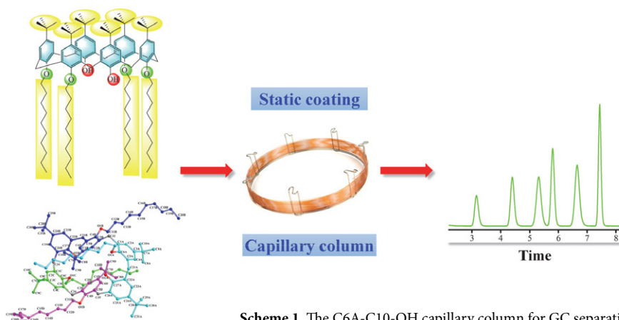
Scheme 1. The C6A-C10-OH capillary column for GC separation.
