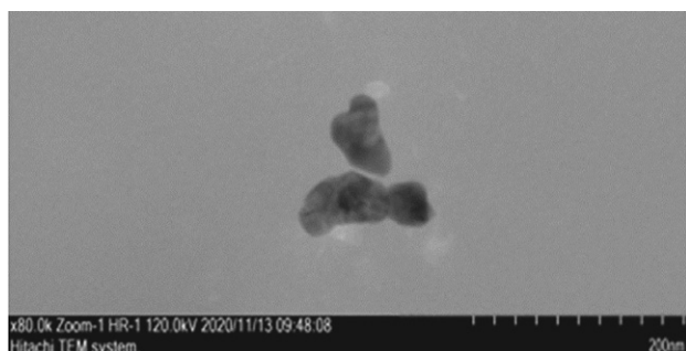
Figure 1. Transmission electron microscopy image of CuO-NPs.
