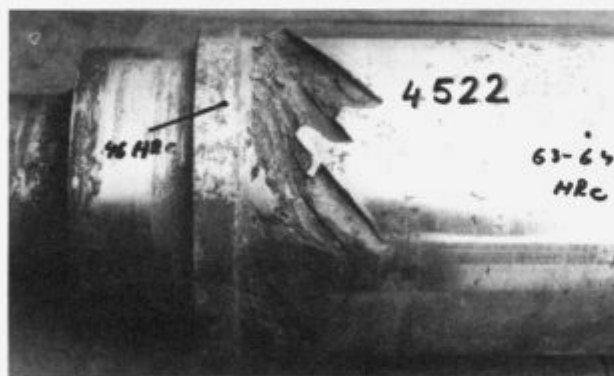
Slika 12: Valjanje tik ob robu valja iz jekla OHV 4 Figure 12: Rolling at the end of working roll surface of steel OHV 4
