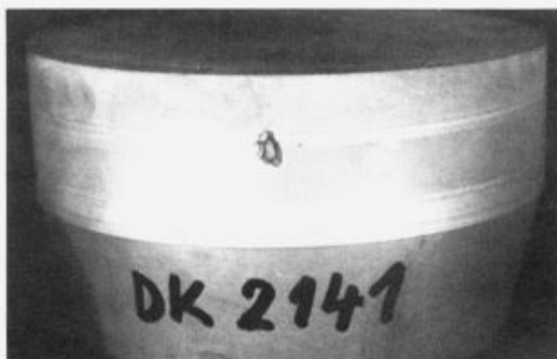
Slika 13: Vtisnjeni delec na valju iz jekla OHV 4 Figure 13: Foreign particle in surface of roll of steel OHV 4
