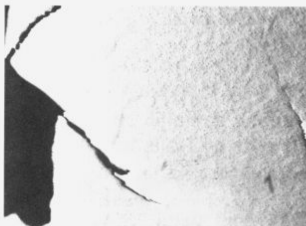
Slika 4: Mikrorazpoka v mikrostrukturi jekla BRM 2, pov. 100x Figure 4: Microcrack in microstructure of steel BRM 2, Mag. 100x
