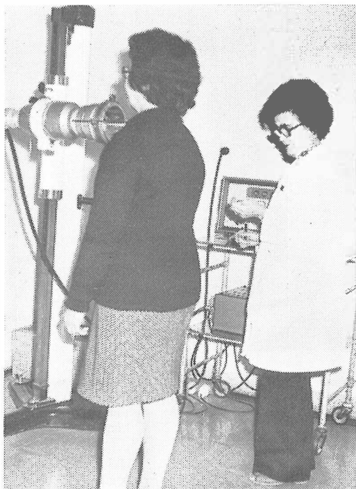
Figure 5a. Thyroid uptake set since 1962 with a home made collimator consisting of lead rings. Designed in the Institute of Nuclear sciences "Boris Kidrič" Vinča, Belgrade.
