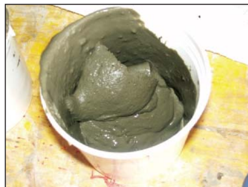
Figure 5. Grout mix after hardening.
