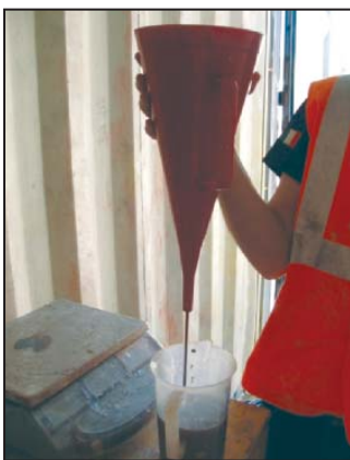
Figure 4. Execution of Marsh cone test.
