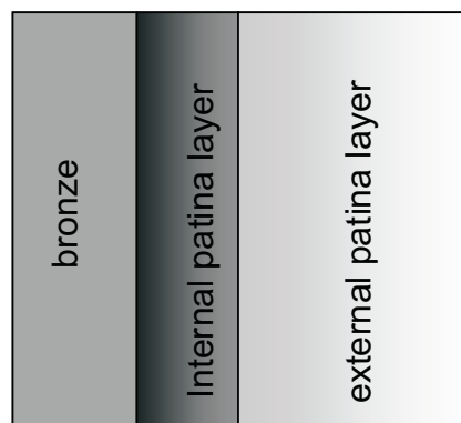
Figure 4: Schematic presentation of patina layers on bronze Slika 4: Shematska predstavitev plasti patin na bronu
