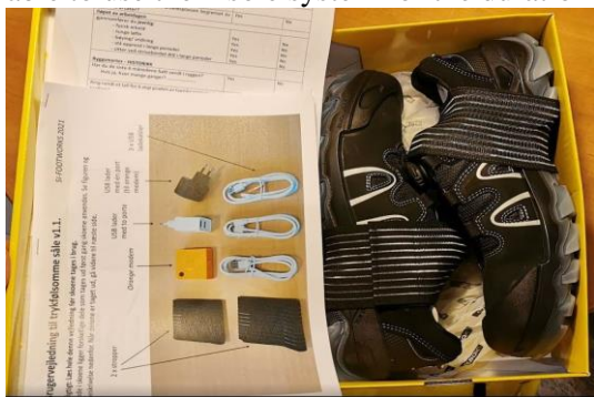
Figure 4. A picture of the entire set of shoes, insoles, gateway, accessories and instructions how to use the insoles, where care should be taken due to fragile parts as well as charging and how to switch on and off the system.
