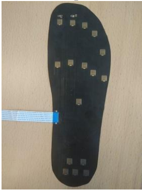
Figure 2. Insole Showing Array of Sensor Terminals
