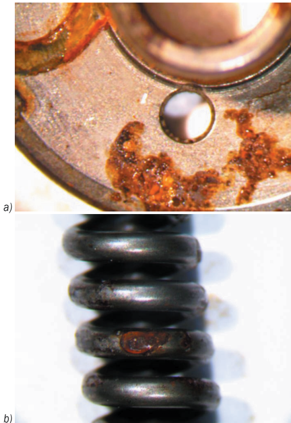
Fig. 5. Corrosion of Bosch fuel injector armature unit; a) disc plate and b) insert spring
