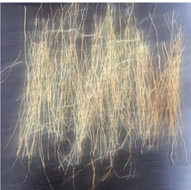
Figure 2: Extracted inflorescence fibre
