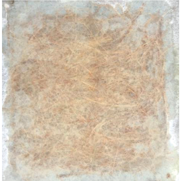
Figure 3: Fabricated glass/inflorescence hybrid composite sample
