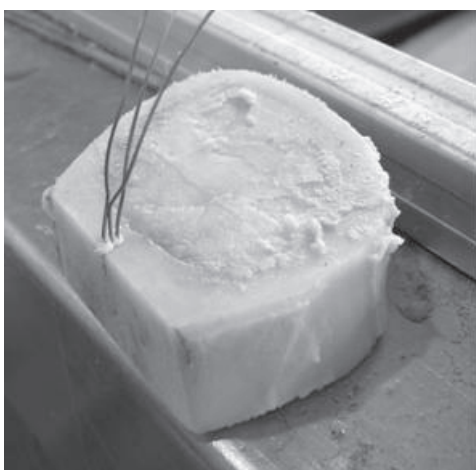
Fig. 2. Preparation of the hollow bone segments (specimens)
