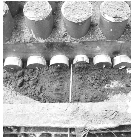
Figure 7: The installations of the thermocouples while molding casting no. 2
