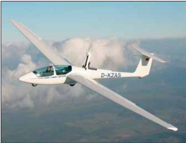
Figure 4. ASK 21 Mi, glider with self launching capability showing its extended propeller. Picture with kind permission of Alexander Schleicher GmbH & Co. Flugzeugbau [Alexander Schleicher GmbH & Co]
