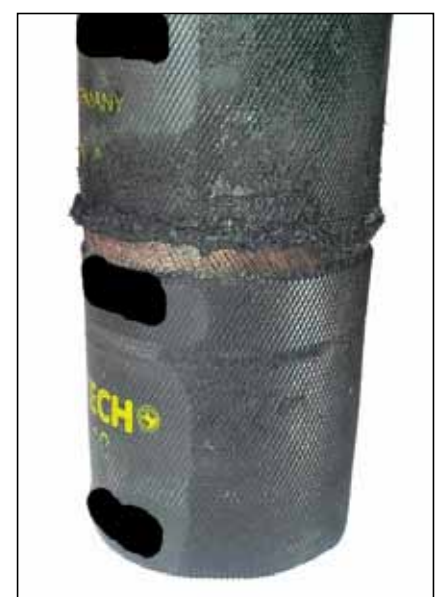
Figure 4. Wear of the bellow
