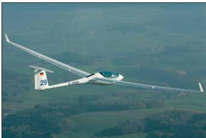
Figure 3. ASW 29 high performance motor glider with its propulsion system retracted. Picture with kind permission of Alexander Schleicher GmbH & Co. Flugzeugbau [Alexander Schleicher GmbH & Co]
