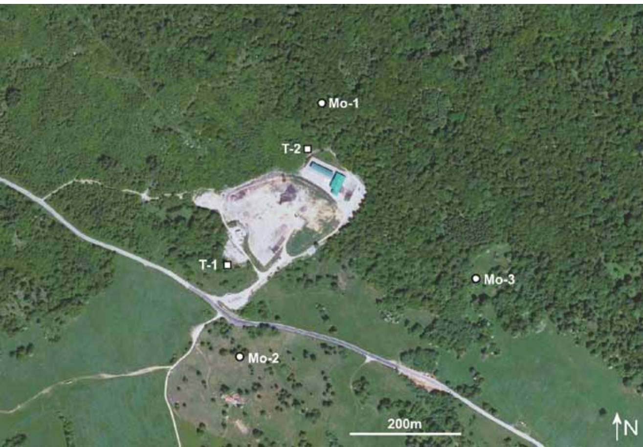
4 Odlagališče Mozelj s točkama injiciranja T-1 in T-2 ter vrtinami za monitoring Mo-1, Mo-2 in Mo-3 (topografska osnova: ARSO 2010). The Mozelj landfill with injection points T-1 and T-2 and monitoring boreholes Mo-1, Mo-2, Mo-3 (topographic base: ARSO 2010).
