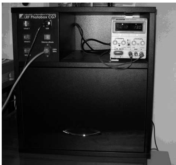
Figure 1: Developed device for measurement of luminance of symbols on car switches.
