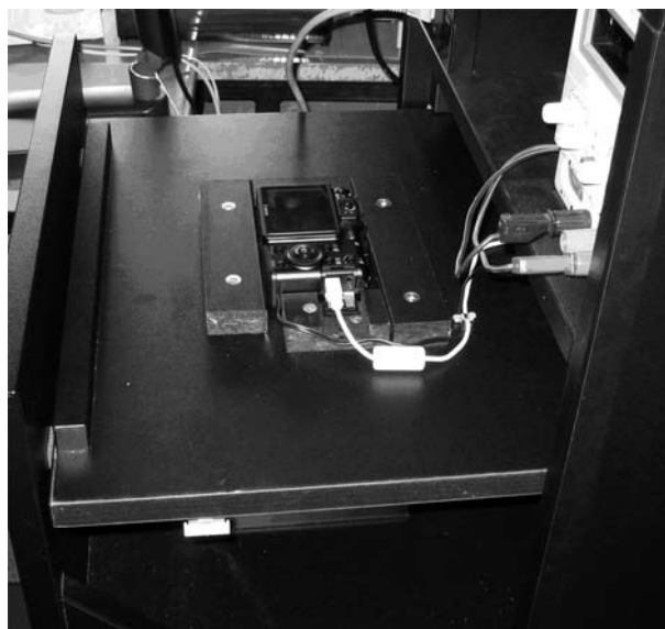
Figure 3: Digital camera is positioned on the top of the measured specimen.
