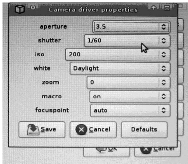
Figure 7: Settings which are send to camera before picture is taken.
