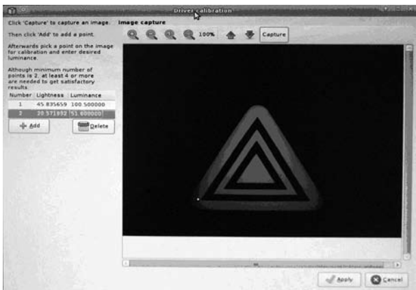
Figure 5: Part of the software for calibration of the measurement system.
