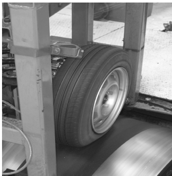
Fig. 5. Tire and drum during cornering test
