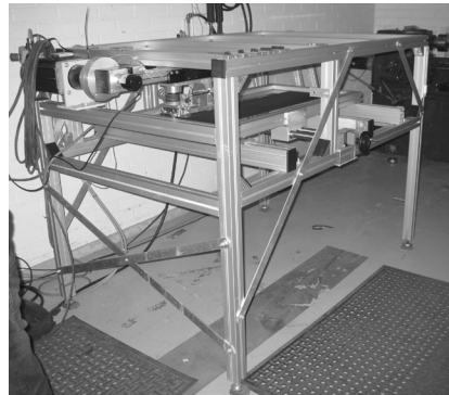
Fig. 8. Mini- \mu -road, linear friction tester that enables sliding of rubber specimens over various kinds of surfaces
