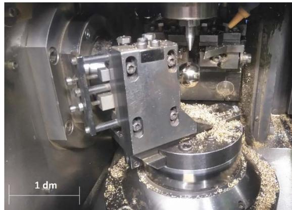
**Fig. 1** Experimental setup for diamond fine turning of CuZn40Pb2
