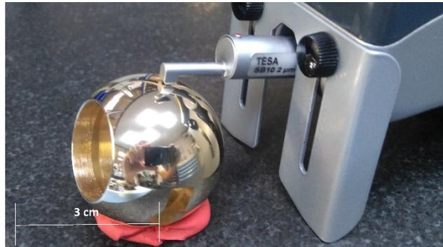
**Fig. 2** Surface roughness measurements
