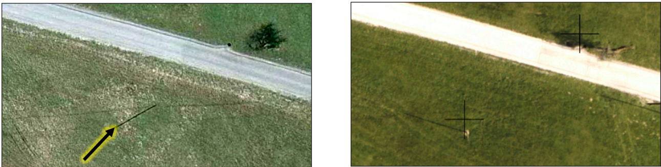
Figure 10. The left image shows a 2004 photo where the position of the power line pole on the ground (arrow) is clearly visible. The right image shows a 2014 photo of the same pole marked with a cross. The displacement is obvious and is 2.1 m.
