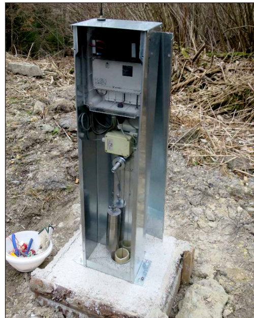
Figure 6. On the left, searching for a movement detector location through a clearly pronounced lateral crack. Right, measuring station to monitor the movement in the borehole. Station MS1.
