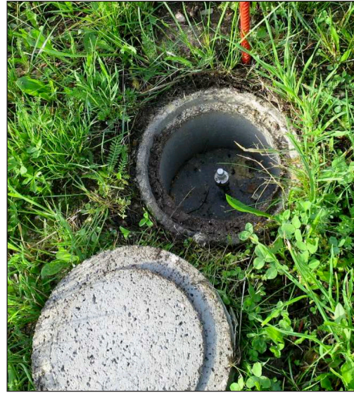
Figure 5. On the left, a measuring column on stable ground, in the background Leskovica, where a measuring prism is placed on the bell tower. Right, polygon point in the ground under a protective cover.
