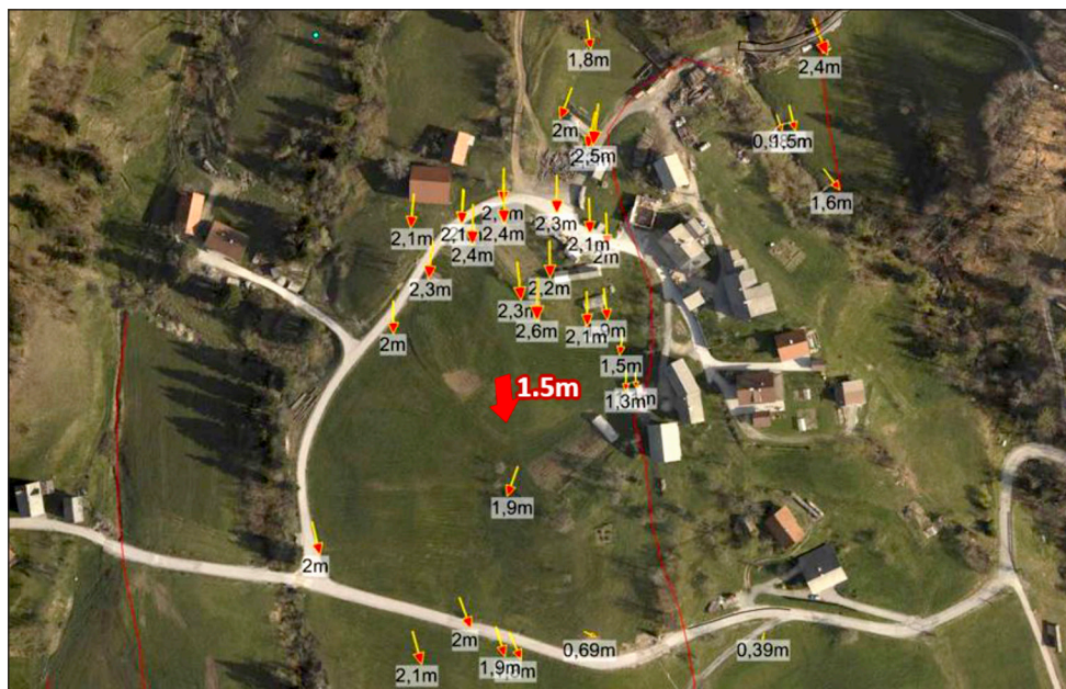
Figure 11. Graphical display of the displacements between 2005 and 2014.
