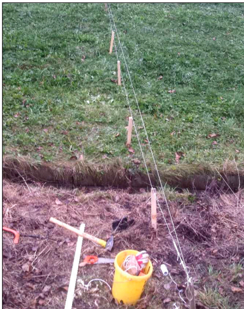
Figure 6. On the left, searching for a movement detector location through a clearly pronounced lateral crack. Right, measuring station to monitor the movement in the borehole. Station MS1.
