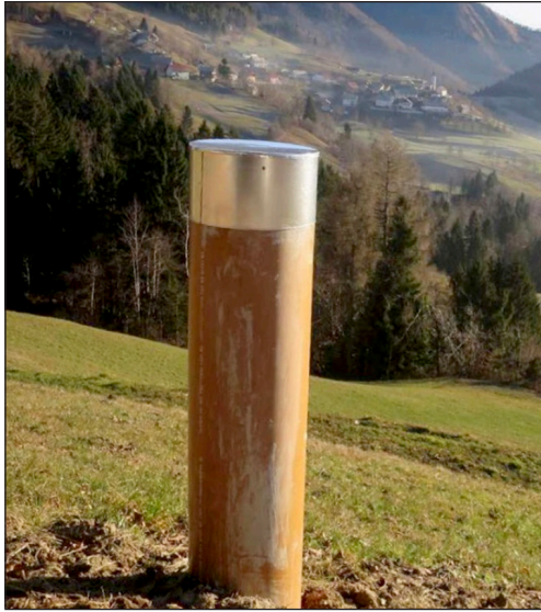
Figure 5. On the left, a measuring column on stable ground, in the background Leskovica, where a measuring prism is placed on the bell tower. Right, polygon point in the ground under a protective cover.
