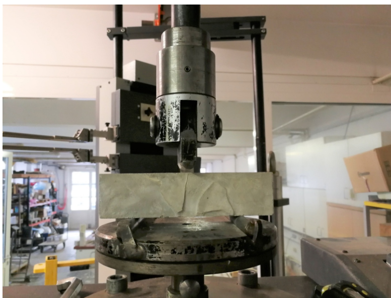
Slika 3.5: Meritve upogibne natezne trdnosti betona. Figure 3.5: Measurements of the flexural strength of concrete.
