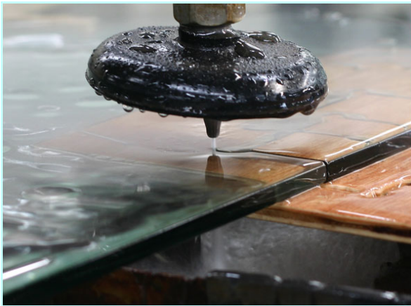
Figure 7. Cutting of glass. AWJ was turned on outside of the workpiece.
