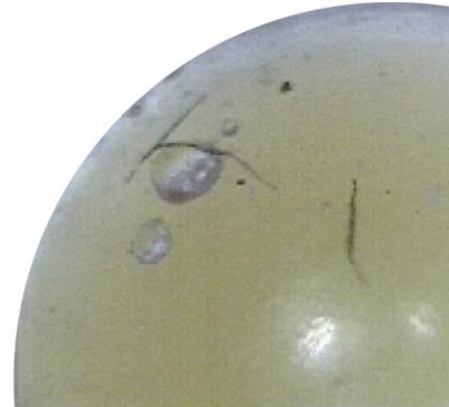
Figure 12 The fractures and deformities on the phosphor layer
