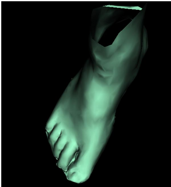
Figure 10. 3D mesh generated from point cloud acquired using hand held laser line projection based device after performed denoising procedure
