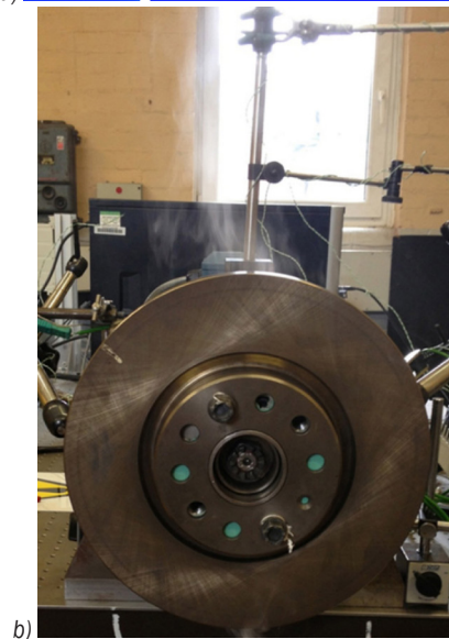
Fig. 10. Ventilated disc: a) CFD air velocities, and b) flow (smoke) pattern using smoke generator
