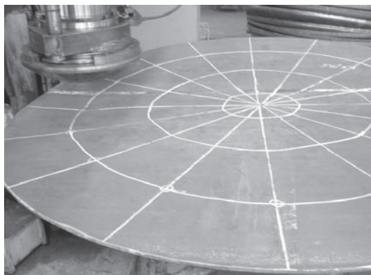
Fig.5. Incremental forming of spherical tank end
