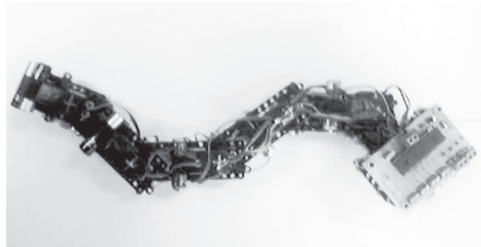
Fig. 9. Shape of a snake-like robot at phase delay \varphi = 1.5 rad
