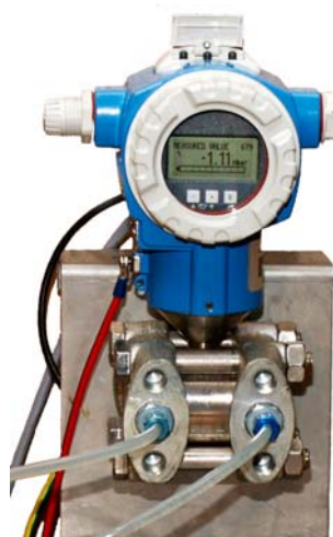
Slika 5.12: Diferenčna tlačna sonda Endress & Hauser Deltabar PMD75 Figure 5.12: Differential pressure sensor Endress & Hauser Deltabar PMD75
