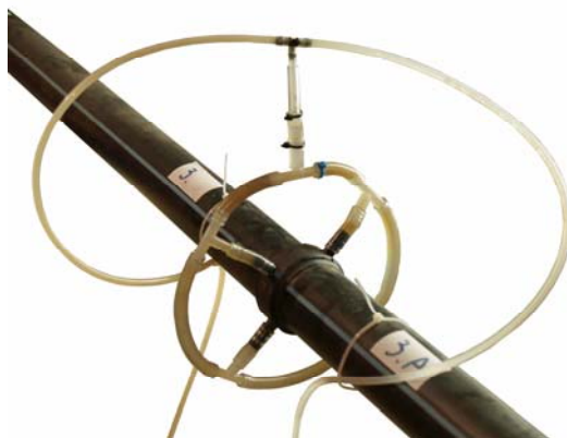
Slika 5.5: Primer namestitve merilnega prereza Figure 5.5: Pressure taps at measuring section
