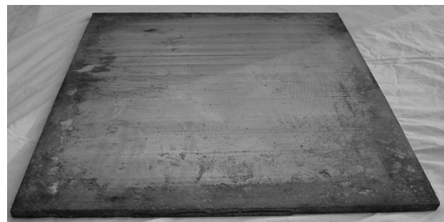
Figure 4: Specimen for sample making with the dimensions of 680 mm × 580 mm × 13 mm
