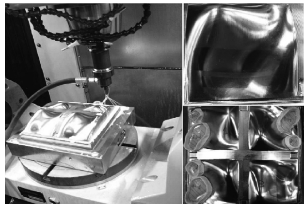
Figure 1: Free-form surface and its machining 1
