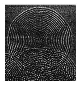
**Figure 7.** Actual high resolution electron microscope image of an onion-like spheroidal carbon particle. Flattening of the shells is most obvious in the arcs between 8 o'clock and 11 o'clock. Image from Daniel Ugarte.
