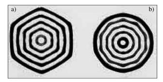
**Figure 6.** Simulated high resolution electron microscope images of a carbon particle consisting of 5 concentric Fullerene cages seen along two different axes; a) The left hand image shows 6-fold symmetry whereas b) the right hand image shows 10-fold symmetry.
