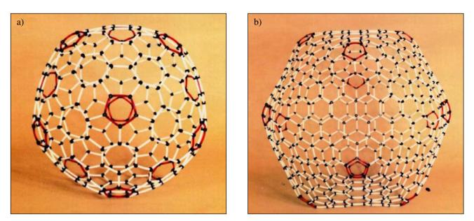
**Figure 2.** Photographs of molecular models of the Giant Fullerenes  $C_{540}^{40}$  (a) and  $C_{960}^{60}$  (b). The models were based on the Goldberg polyhedra. Notice that as the cages become larger the icosahedral symmetry of the structure becomes more and more obvious as the overall shape becomes less spheroidal and more polyhedral.
