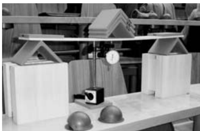
Slika 3: Upogibni preizkus preizkušanca iz lesa na FA. Bending test of a wooden sample at the Faculty of architecture.
