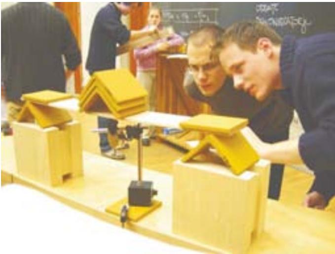
Slika 1: Upogibni preizkus na posameznem preizkušancu iz lesa v predavalnici Fakultete za arhitekturo (Foto: Edo Wallner). Bending test on a particular wooden sample carried out in the lecture hall at the Faculty of architecture.
