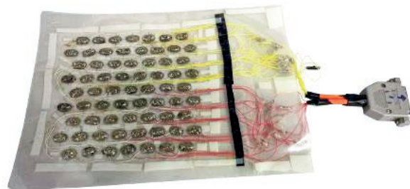
FIGURE 2. Prototypes of the flexible electrode: (A) device with diameter 8 cm with hexagonal electrode disposition, (B) removable needles inserted in electrical connection and (C) square device 15 x 15 cm with hexagonal arrangement of conductive guides highlighted.
