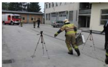
Slika 7: Test hitrosti prenašanja bremen – kaset (B, C in VT) (Bračič in Vodičar, 2010)
