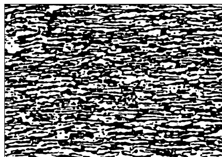
Fig. 5. Binary image of rolled stainless steel in a longitudinal section. The light phase is ferrite, the black phase is austenite. From Ohser and Mücklich (2000).
