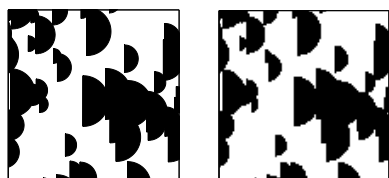
Fig. 3. Boolean model with non-isotropic grains. Left: a realisation of the model on the unit square. Right: a digitised image of the realisation with resolution 100 \times 100 .
