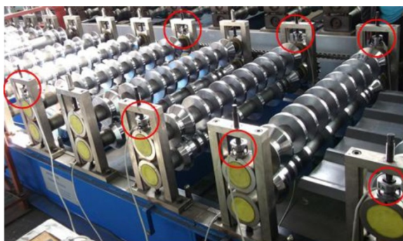
Fig. 4 Roll forming production line used in experiments
