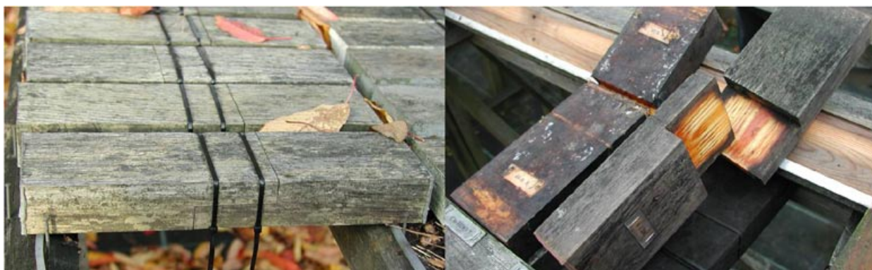
■ Slika 4. Lap-joint terenski test (foto: Miha Humar) Fig. 4. Lap-joint field test (photo: Miha Humar)
