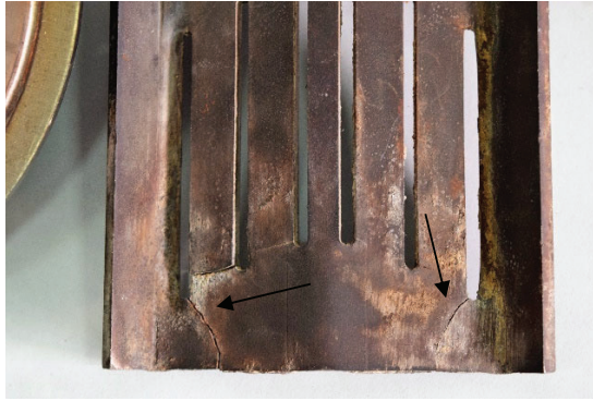
Figure 5: Hot cracks as a damage of the steel grille
