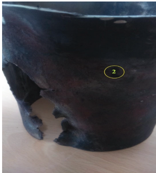
Figure 7: Target point (number 2) for manual measurement of chemical analyses of real steel tube (tubular combustion chamber)
