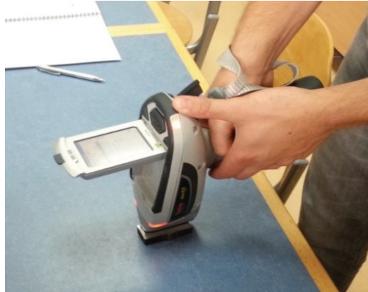
Figure 6: Manual measurement of chemical analyses of steel tube (tubular combustion chamber) with X-ray fluorescence spectrometry (XRF) using an X-ray fluorescence spectrometer
