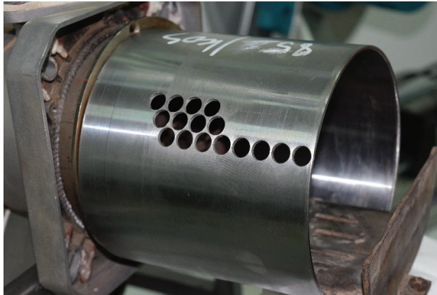
Figure 10: Cr-Mo steel tube with damaged surface (16 holes)
