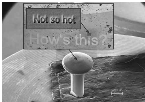
Figure 1: Feynman's experiment: "High school competition". The "o" letters in the smallest box have an internal diameter less than 400 nm.
