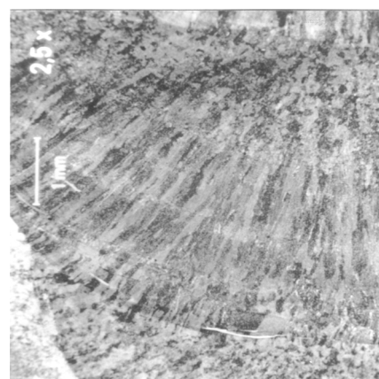
Figure 3: The re-heated and as-welded region within a welded pass, \times 20
