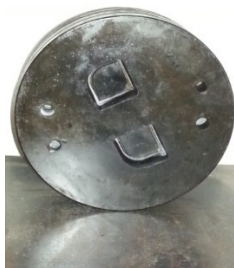
Fig. 10 Corner section die after assembly
