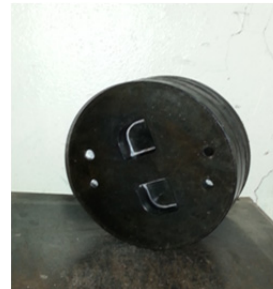
Fig. 11 Corner section die after grinding process
