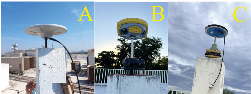
Figure 4: Antennas and stations used for the experiment. A) CULC CORS station from INEGI. B) GEOMAX ZENITH25. C) ASH701975.01A
