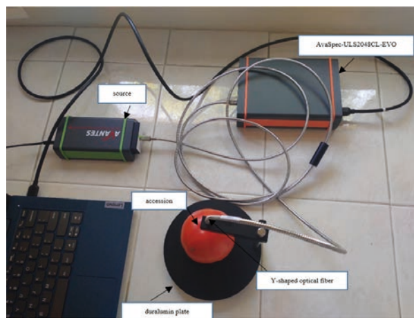
Figure 1: Accustomed aspect of the experimental installation used by fluorescence spectroscopy
