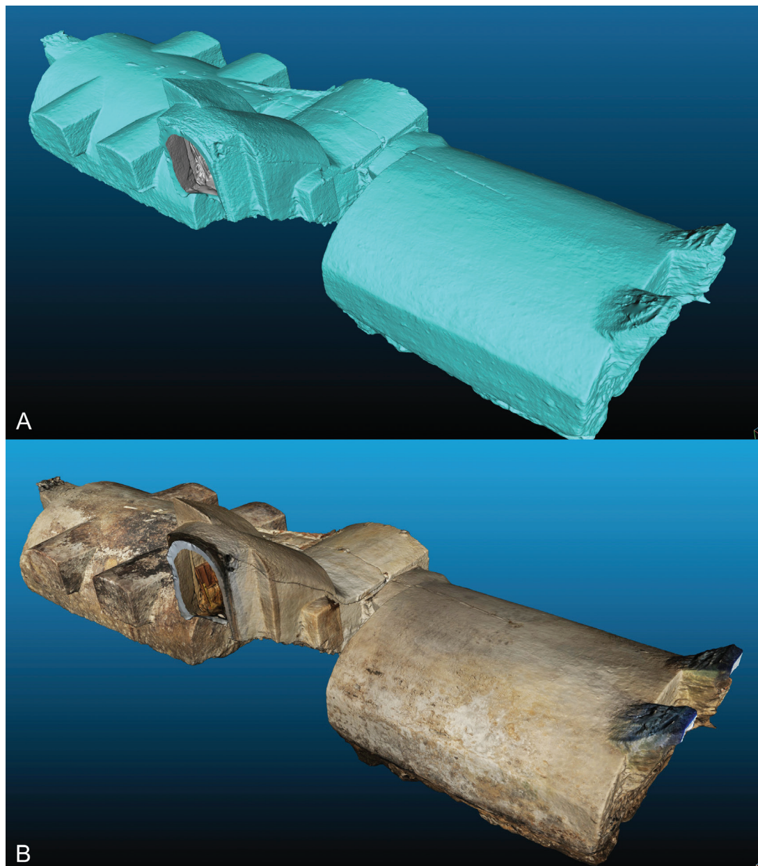
Figure 69. Rajec (Slovakia). Burgess house (16 th century), cellar. IBM. Isometric views of the exterior. A: shaded 3D model, B: textured 3D model.
