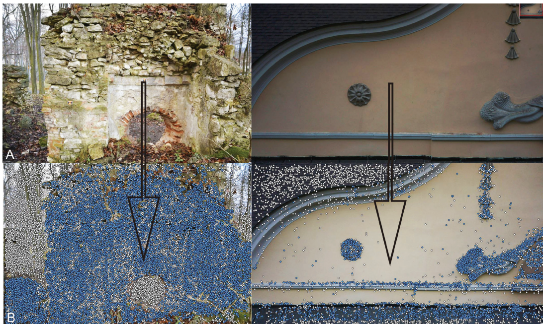
Figure 72. Distribution of SIFT points (key points) detected by bundle adjustment. A: raw stone structure, B: flat facade covered with single-colour fine plaster.
