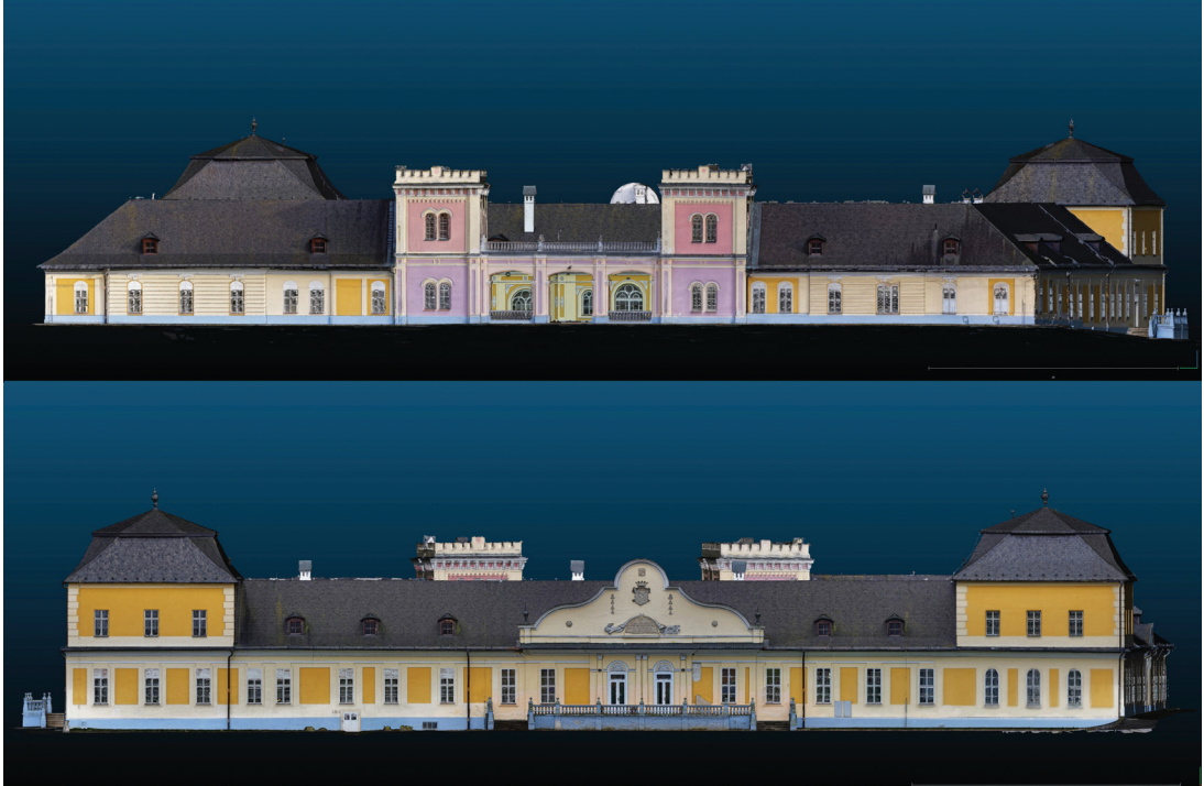
Figure 50. Žehra, Hodkovce (Slovakia). Manor house (18-19 th century), exterior. lBM in combination with TLS. Ortho-views of the facades.
