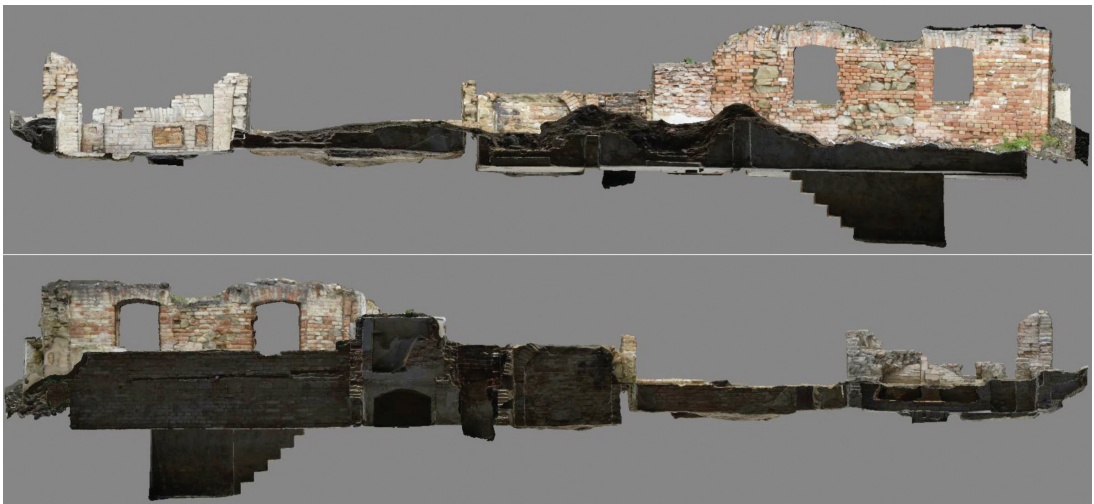
Figure 23. Senec, Synagogue (Slovakia). Remains of the economic section of the synagogue. Cross-section documentation derived from the 3D model.
