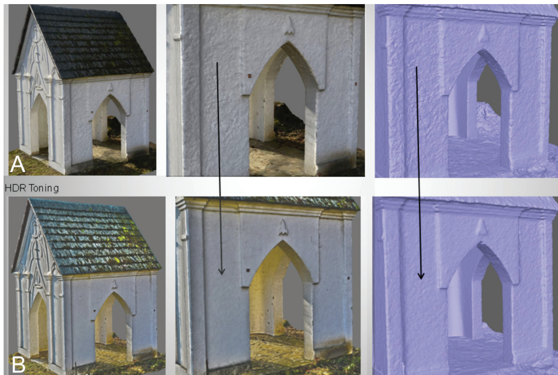
Figure 74. Example of HDR filtering/toning of photos leading to better quality of the final 3D model (mesh) on one hand, and false colour information on the other. A: mesh built from photos with default settings, B: mesh built from HDR-toned photos.
