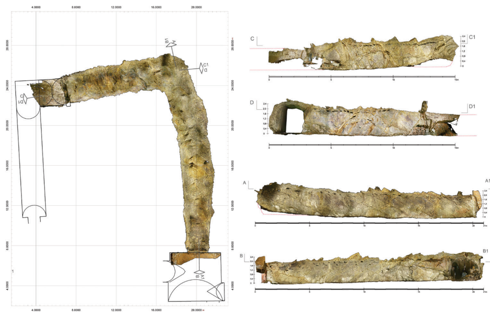
Figure 65. Banská Belá (Slovakia). Mining site, 15 th century. Example of 2D documentation derived from the 3D model.
