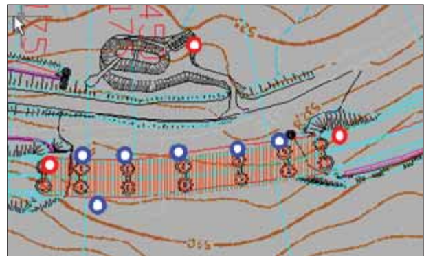
Figure 6. Example of different observation points on a viaduct.
