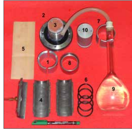
Figure 3. Basic elements for the specimen preparation: 1) lifting device of the three-part mould; 2) fixed lower base; 3) porous stone; 4) three-part split mould; 5) latex membrane; 6) O-Ring; 7) O-Ring stretcher; 8) extension of three-part mould; 9) 500-cm 3 beaker with de-aired water; and 10) loading head.
