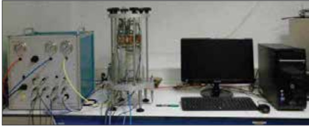
Figure 1. Resonant-column apparatus manufactured by Wykeham Farrance.
