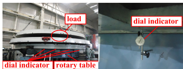
Fig. 11. Bearing capacity experiment setup
