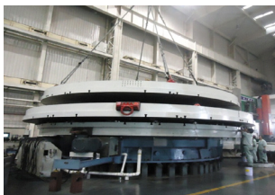
Fig. 9. The optimized hydrostatic rotary table
