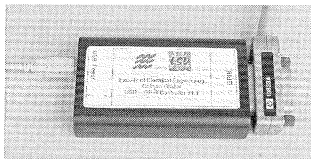
Fig. 3: The controller with connected cables
