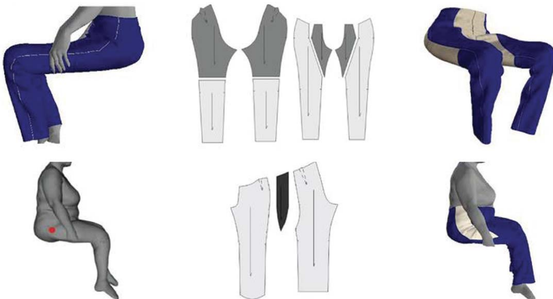
Figure 8: Developing trouser patterns for people in the sitting position [65]
